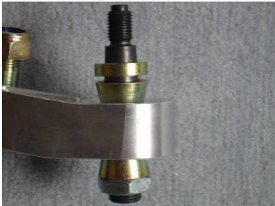
The control arm's outer joint is mounted using conus bearing as shown left. The mounting position can be adjusted using the supplied spacer. Installation of the spacer is not absolutely required.
