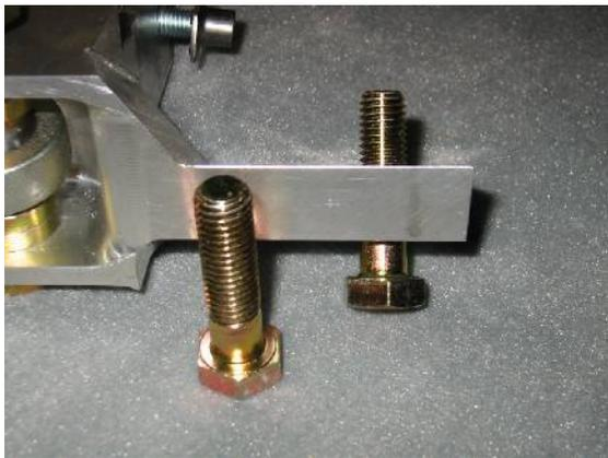
Use the supplied screws M12x1.5 to attach the other points of the radius arm mount to the chassis. The existing threaded holes in the chassis must be enlarged.
