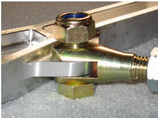
Installation of the fork on the radius arm and attachment to the control arm is shown on the left.
