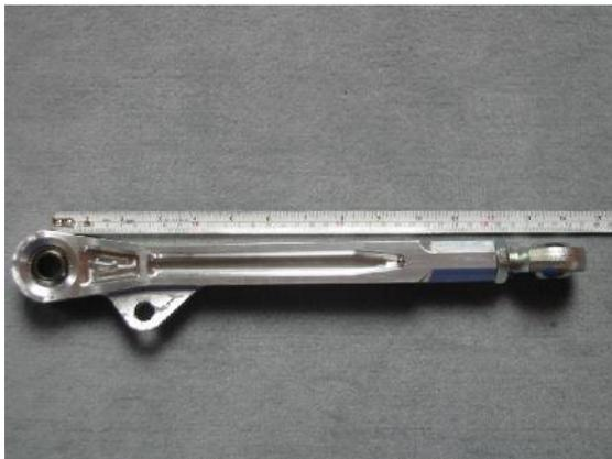
In order to achieve the stock wheel position, the control arm is adjusted to a length of 340 mm measured center to center between the bearing ends.
