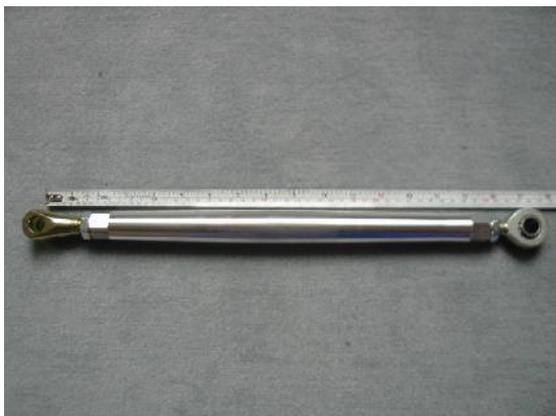
In order to achieve the stock wheel position, the radius arm is adjusted to a length of 435 mm measured between the center of the fork bolt hole and the rod-end center.
